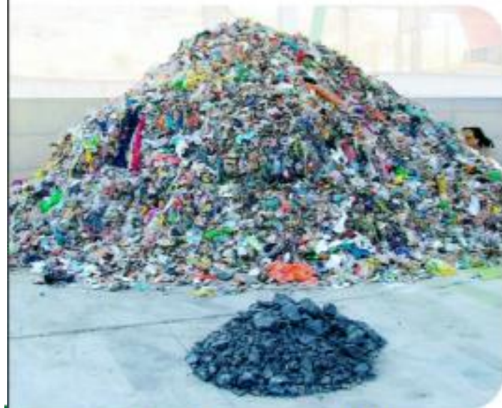
A waste pile and the corresponding inert glass aggregate after treatment (close-up above)
