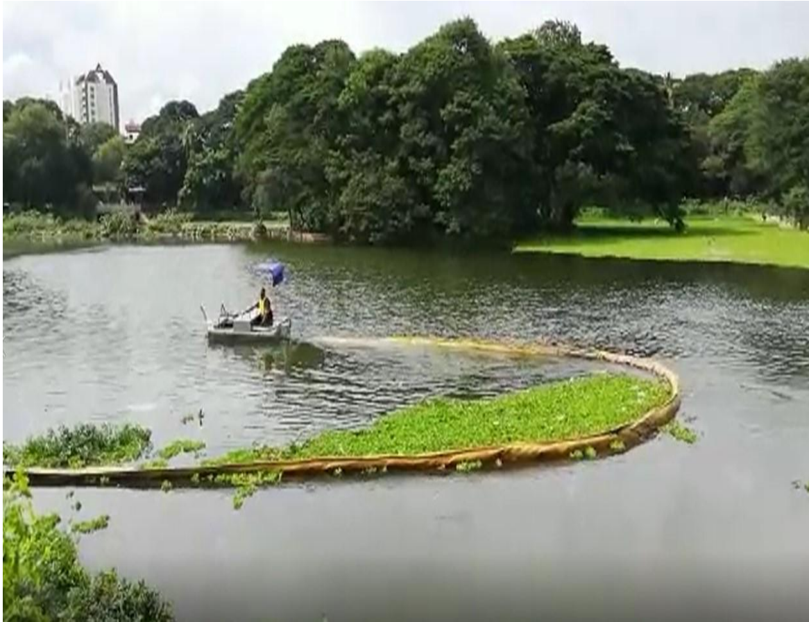
Tandem Sweeping of lakes with waterjet propelled boats
